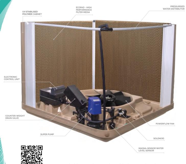
Scan to watch video - CoolBreeze Airconditioning - How it works
