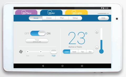
The home screen gives you an overview of the air-conditioning status. Adjust the temperature from this screen, or tap through to zones to fine-tune the airflow to every room.
